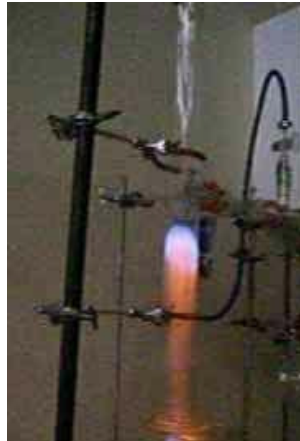
Figure 3.9: Photo of methane-air flame color without addition of inhibitors.
