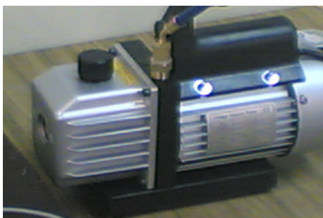
Figure 3.3: Picture of vacuum pump used in experimental setup.
