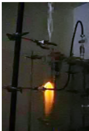
Figure 3.10: Photo of methane-air flame color with addition of CO 2 .
